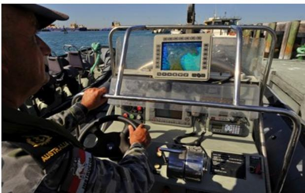
The 9LV SAT is positioned within easy reach of the boat's coxswain. It uses a touch screen, big buttons and a simple screen layout to help crew workload in a rough and stressful environment.
